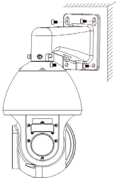
7. Pull the composite cable from the dome through the wall mount and pull it out of the other end of the wall mount bracket.
