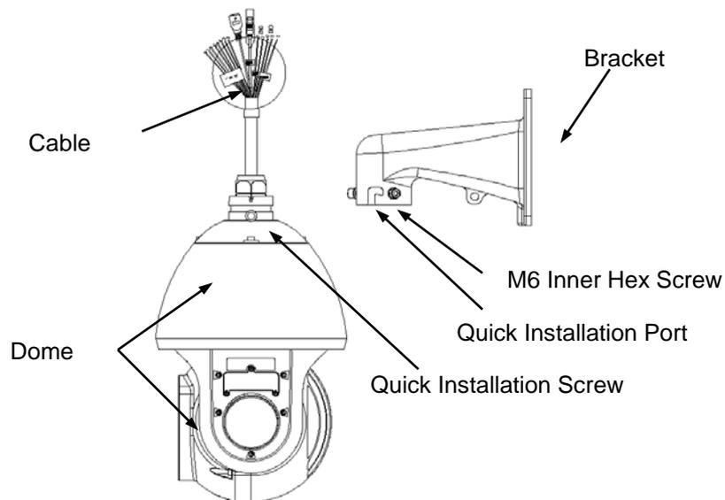
9. Insert the quick installation screw into the port, then move the dome towards the wall to seat the dome in the wall mount.
