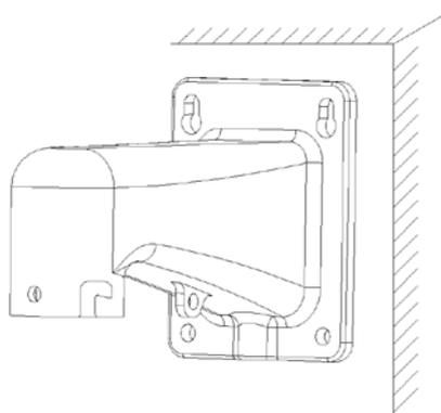
3. Pre-drill the four perimeter holes as marked on the wall for the fasteners, using a drill bit that is no wider than the fastener.
