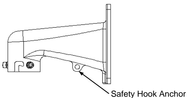
**Caution:** Make sure to attach the safety hook and ensure that it is securely fastened to the dome and to the wall mount to improve the safety and reliability of the installation.
