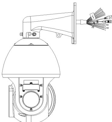
10. Tighten the M6 Inner Hex Screw on the wall mount to secure the dome to the 64FB Wall Mount assembly.
